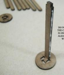
DO NOT GLUE THE STRIP INTO THE CIRCULAR JIG PLATE. THIS IS ONLY TO ENSURE CORRECT ALIGNMENT AND IS REMOVED WHEN THE GLUE DRIES.
